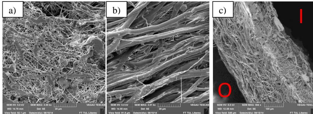
Figure 3: Inner layer of the graft composed of nanofibers with a few deformed fibers and beads (a) and outer layer composed of oriented microfibers (b), scale bars 20  $\mu\text{m}$ . Cross section of double layered PCL graft composed of nanofibers in the inner side (I) and microfibers in the outer side (O). Scale bar 100  $\mu\text{m}$  (c).
