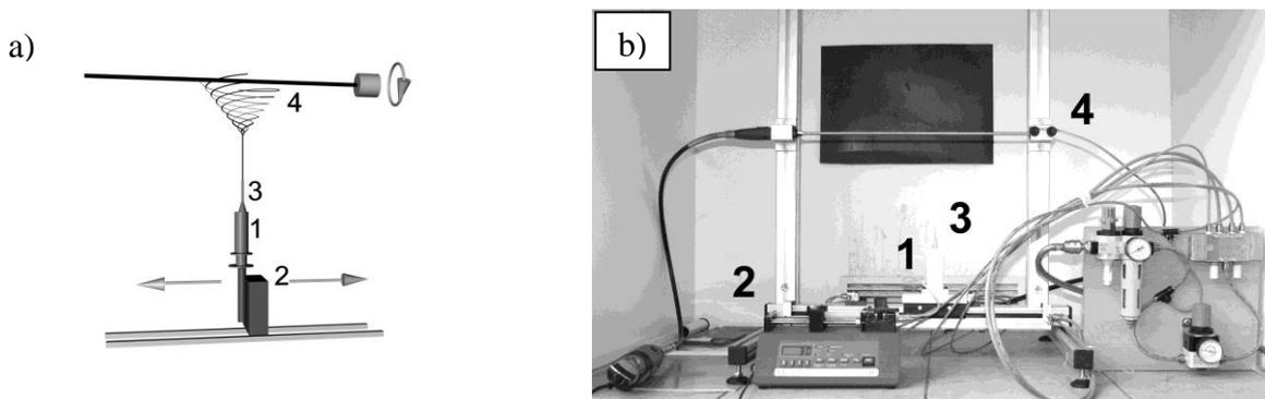
Figure 1: The schema (a) and photo (b) of electrospinning setup used for small diameter vascular grafts. Syringe pump (2) doses polymeric solution in the syringe (1) that is connected to the positively charged needle (3). Forming fibers are collected on the rotating mandrel (4).
