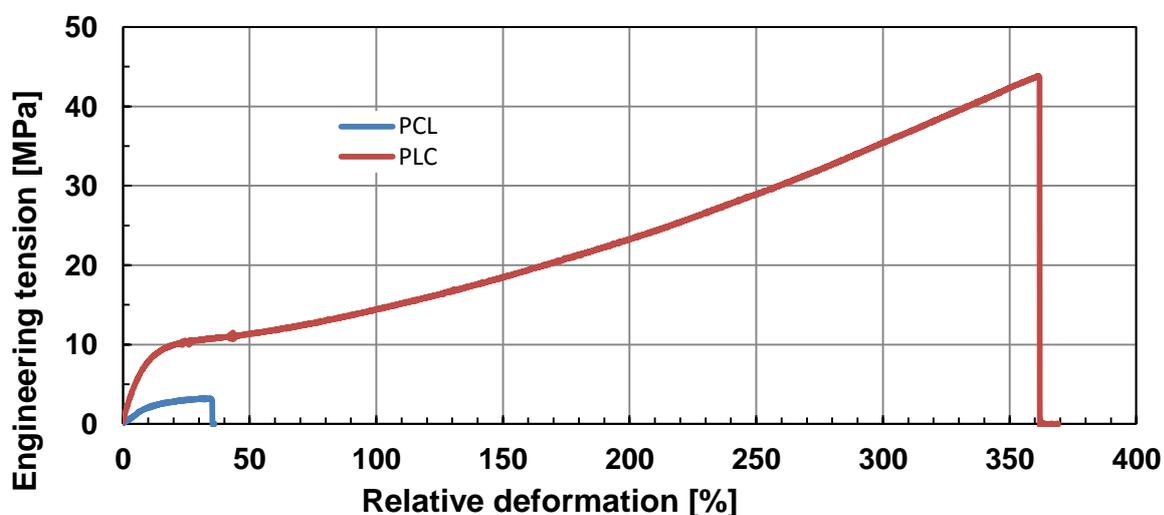
Figure 5: Comparison of stress-strain curves of PCL tubular fibrous layer (blue line, 29  $\mu\text{m}$  thickness) and PLC layer (red line, 29,5  $\mu\text{m}$  thickness).
