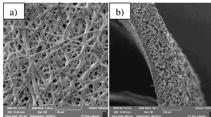
Figure 4: Fiber morphology of electrospun copolymer PLC (a), scale bar 50  $\mu\text{m}$  and cross section of vascular graft made from PLC (b), scale bar 100  $\mu\text{m}$ .
