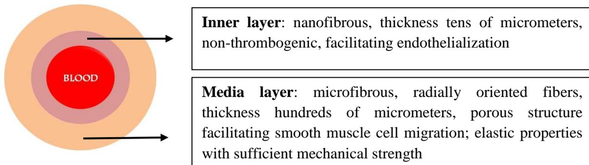
Figure 2: Structural design of double layered vascular grafts.
