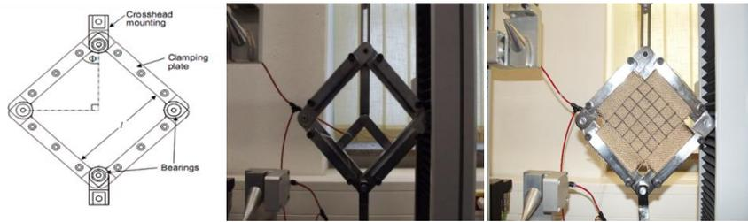
Figure 4: Picture frame fixture design and clamping of sample in fixture
