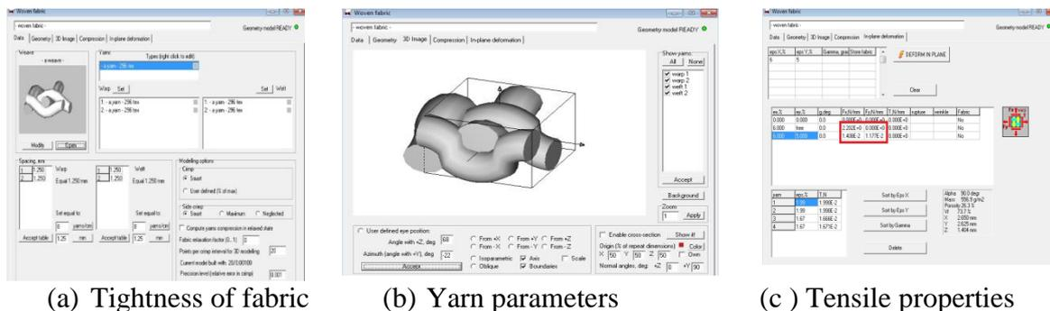
Figure 15: Prediction of tensile properties with WISETEX.
