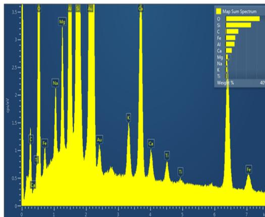
Figure 8: Energy-Dispersive X-Ray Analysis of Basalt
