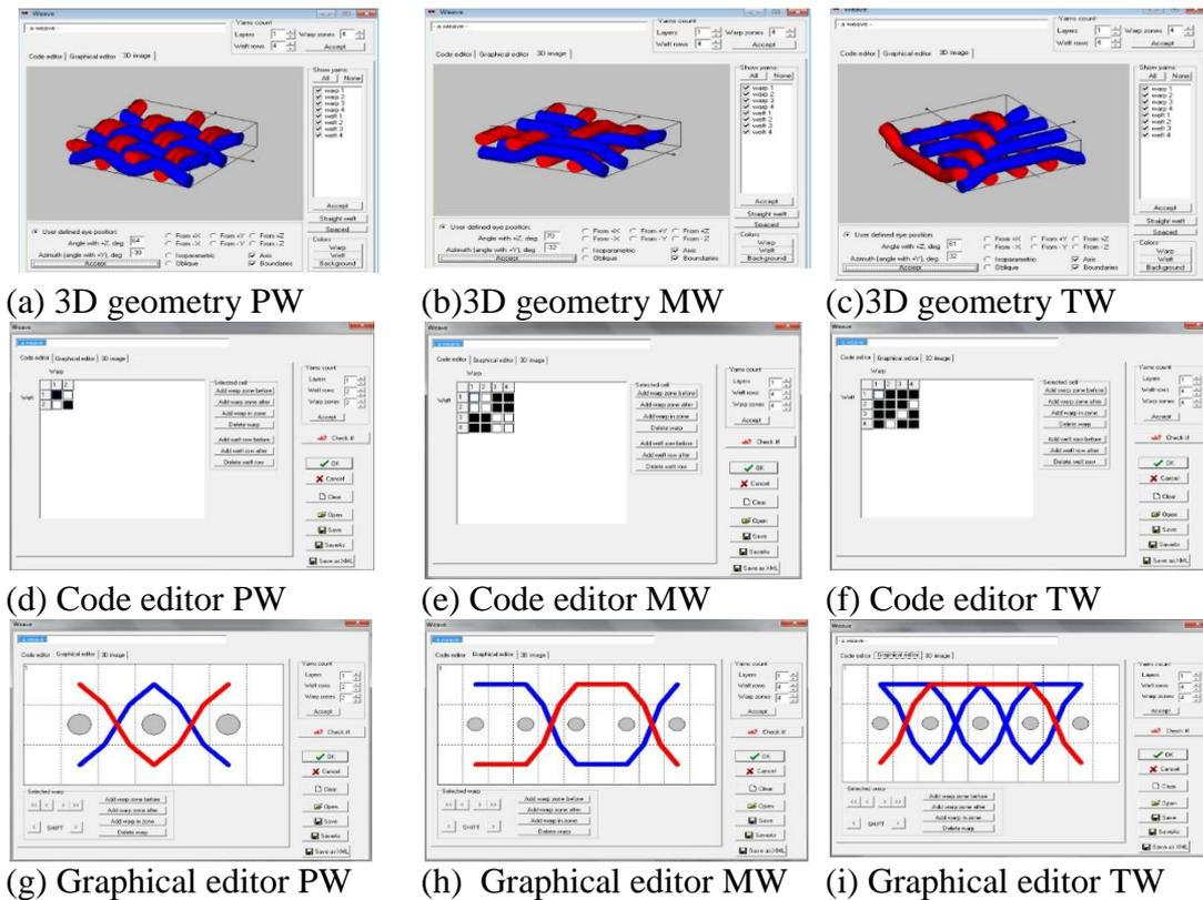
Figure 3 : Weave structure (a-c) 3D image, (d-f) code editor and (g-i) graphical editor.
