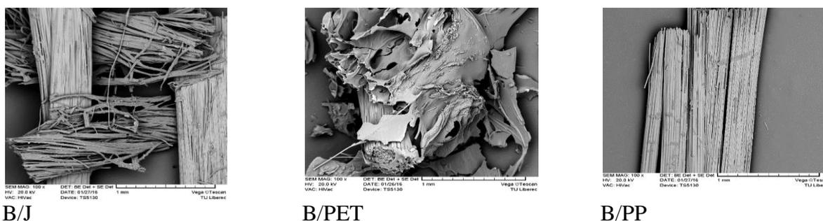
Figure 26: SEM images of hybrid fabrics after TGA.
