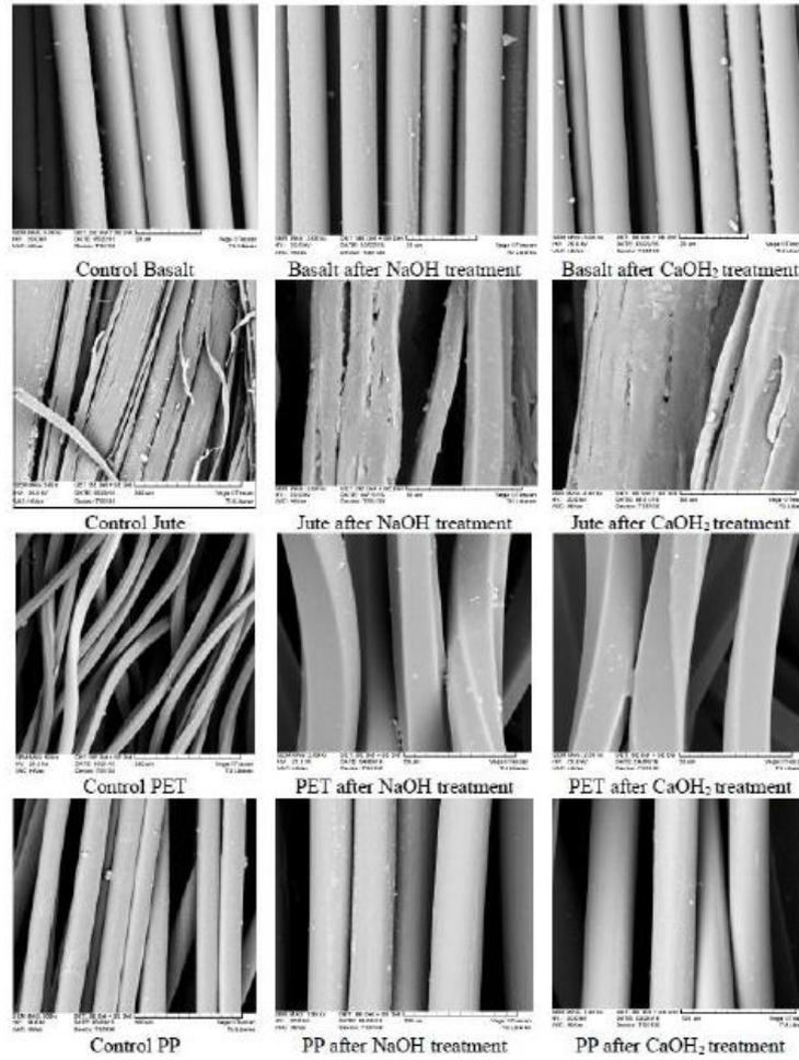
Figure 12: SEM images of fibers after alkali treatment.
