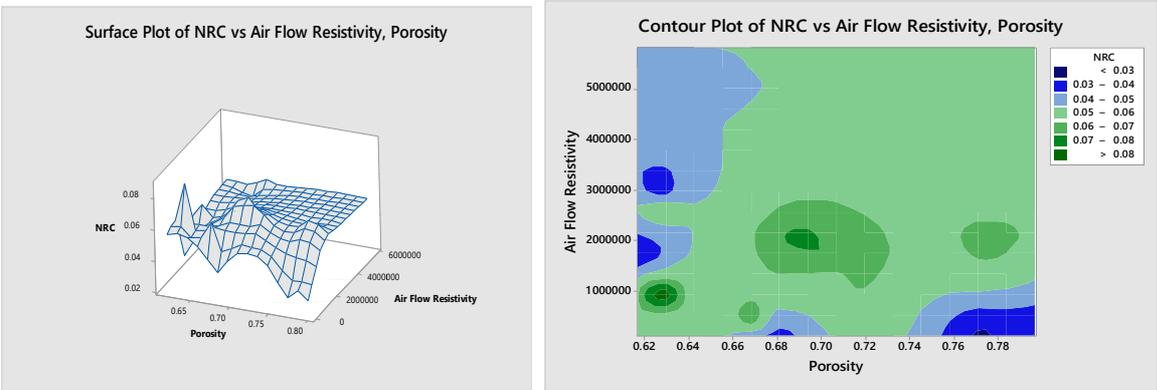
Figure 23: Relationship between fabric porosity, airflow resistivity and NRC. Matt weave structures have highest value of NRC due to more porosity. This phenomenon
