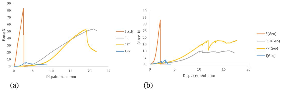
Figure 13: Force vs displacement for yarns in Portland and Geopolymer cement.
