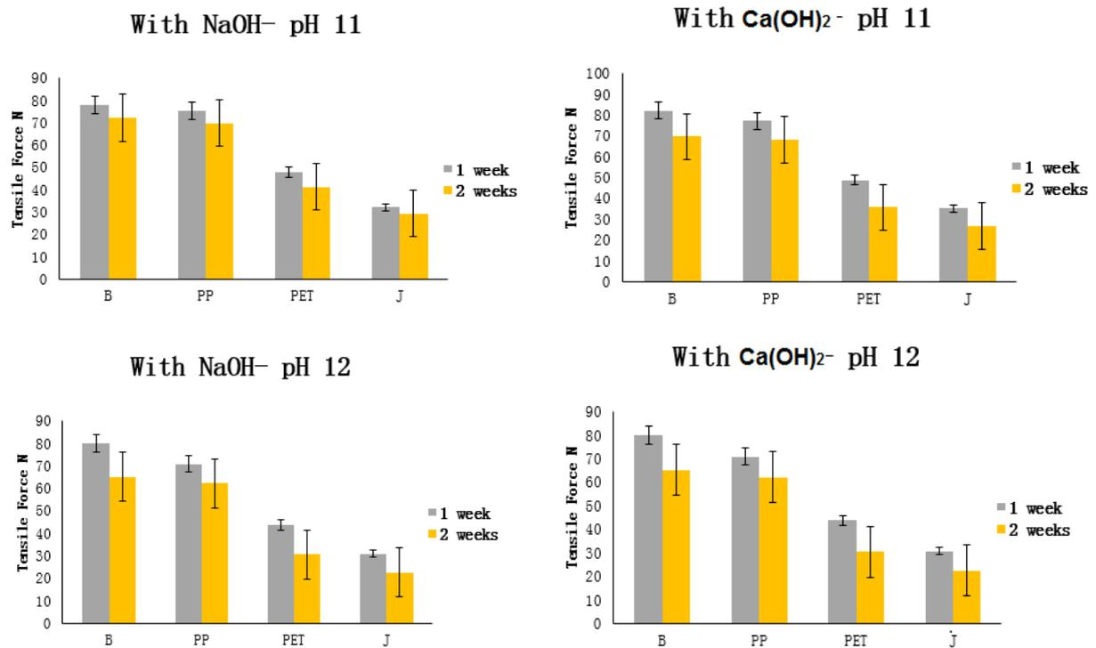
Figure 11: Effect of time on degradation of yarn after alkali treatment.
