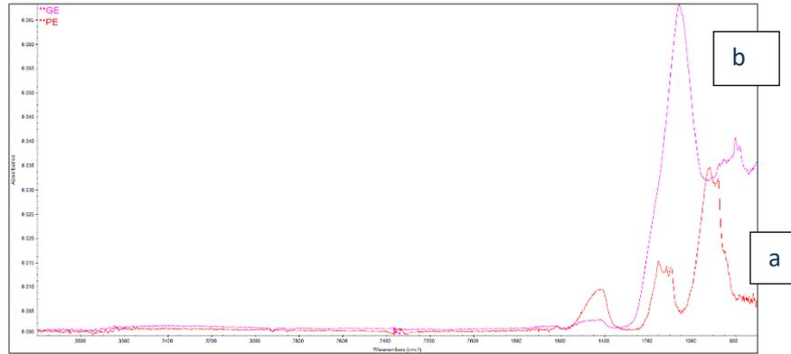
Figure 9: FTIR spectra of used cement materials (a) OPC, (b) GPC.
