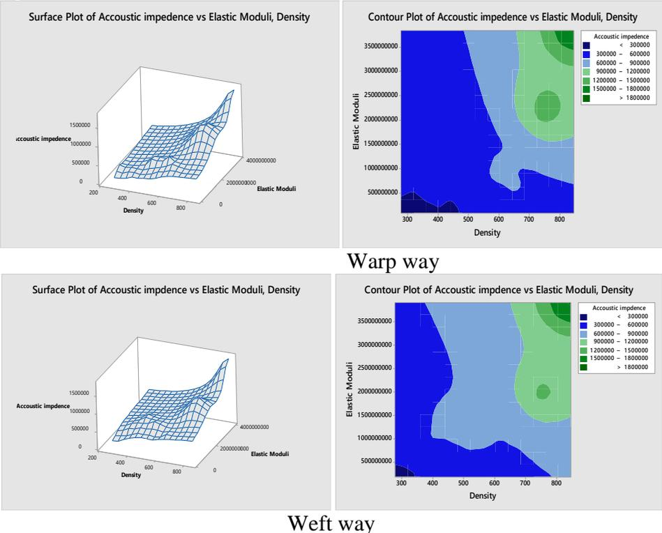
Figure 24: Dependence of specific acoustic impedance on elastic moduli and density of woven fabrics.
