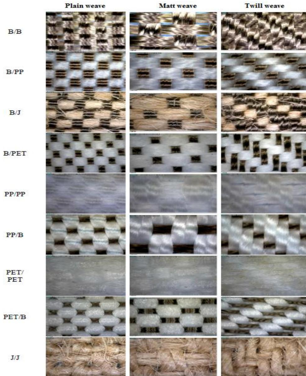
Figure 2: Photographs (Dinolite) of the structures developed with magnification 1280 x1024
