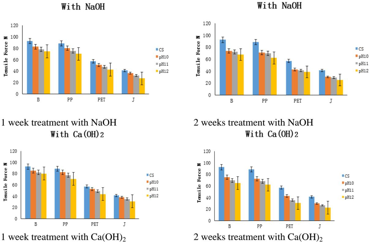
Figure 10: Effect of pH on degradation of yarn after alkali treatment.
