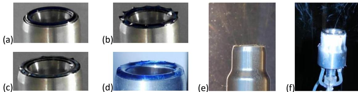
**Figure 6** The record of needleless electrospinning realized by cylindrical coaxial spinning electrode: (a) the core polymer layer formation, (b) the emerging instability on the polymer layer before reaching value of  $E_c$ , (c) Taylor cones, (d, e) DC electrospinning, (f) AC electrospinning (Vysloužilová, 2015).
