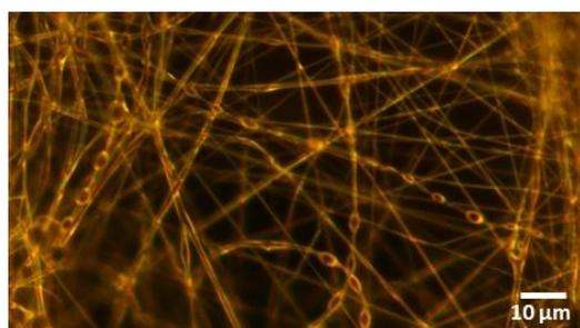
**Figure 23** Core-shell nanofibers with incorporated vegetable oil observed by optical microscopy after 48 hours.
