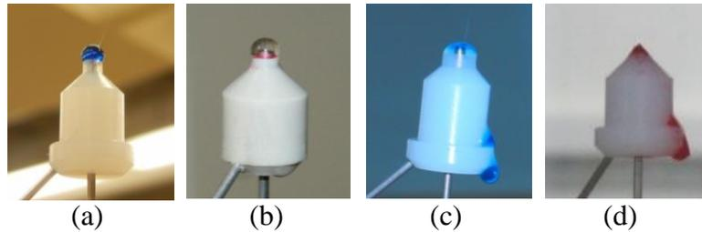
**Figure 11** Developed coaxial needle spinning electrodes with the neck and optimal bi-component polymeric droplet (a, b), the too large of diameter of the spinning electrode orifice caused the droplet slumping (c), the spinning electrode without the neck causes the droplet slumping (d).
