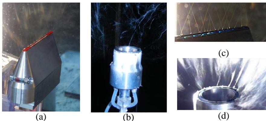
**Figure 19** needleless coaxial electrospinning realized by the cleft electrode (a, c) and by the cylindrical coaxial spinning electrode (b, d).
