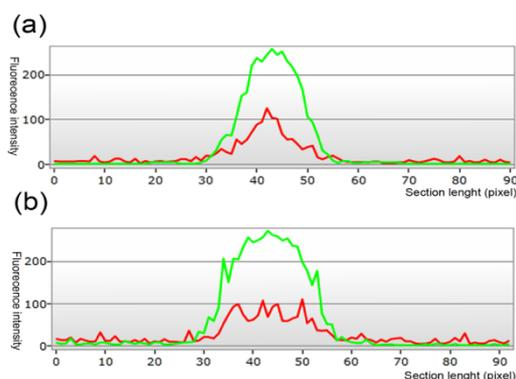
**Figure 28** Signal intensity profiles of fluorophores for core-shell nanofibers realized by (a) the needle coaxial spinning electrode and (b) the weir spinner of the second generation. Fluorescence intensity profiles of FITC-dextran incorporated in the shell (green line) and IgG-PE-AF700 incorporated in the core (red line). Collaboration with Jiří Kula and Matej Buzgo.
