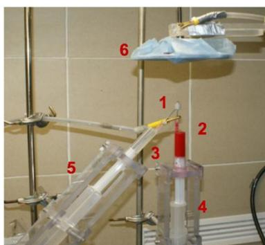
**Figure 3** Laboratory set-up for the needle coaxial: the coaxial needle spinning electrode connected to the HV source with a positive charge (1), the syringe with the core polymer solution (2), the syringe with the shell polymer solution (3), the hydraulic system for the core solution (4) and for the shell solution (5), the collector with the Spunbond nonwovens connected to the HV source with a negative charge (6).
