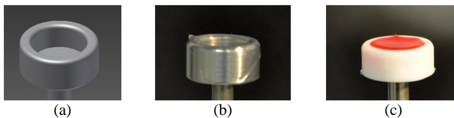
**Figure 12** Pool needleless spinning electrodes: The model of the pool spinning electrode (a), the pool spinning electrode from the electrically conductive (b) and electrically non-conductive (c) material.
