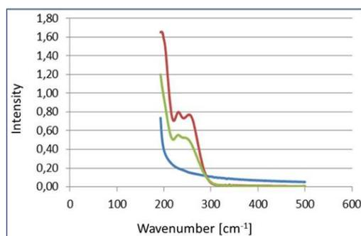
**Figure 25** FTIR spectroscopy of PVA (blue line), disinfection (red line) and core-shell nanofibers PVA/disinfection (green line).
