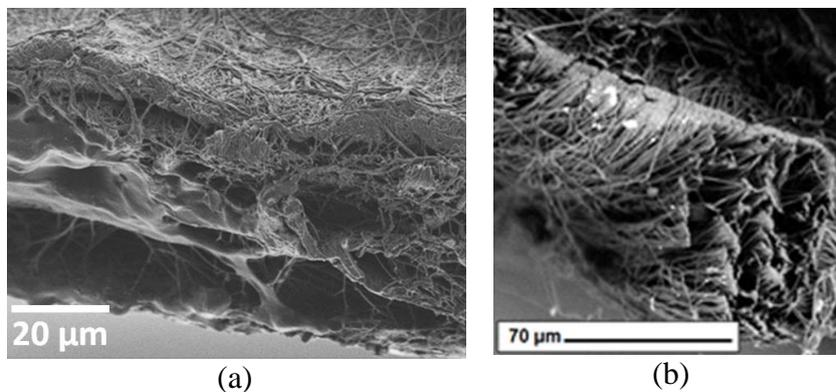
**Figure 21** The cross-sections of the core-shell nanofibers observed using SEM (Zeiss, Germany) (a) and the mechanical cross-section of nanofibrous yarn observed using SEM Phenom (G2, FEI)
