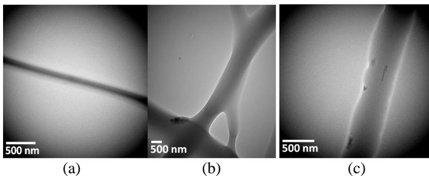
**Figure 24** TEM images of PVA/PVA core-shell nanofibers with Prussian blue (a) and PVA/PVDF core-shell nanofibers with incorporated magnetic nanoparticles (b, c).
