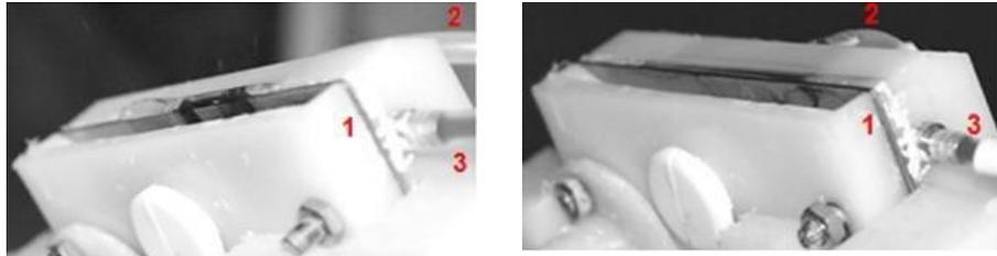
**Figure 1** The weir spinner: polymer two-layer flowing over the spinning electrode (1), feed of the shell polymer solution (2), feed of the core polymer solution (3), (Vyslouzilova, 2010).
