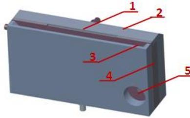
**Figure 16** The Weir spinner of the 2<sup>nd</sup> generation: the chamber for the core polymer solution (1), the chamber for the shell polymer solution (2), the outflow chamber (3), the core polymer feeding tube (4), the shell polymer feeding tube (5), the electrode (6), the holder for HV cord (7), (Vysloužilová, 2011).
