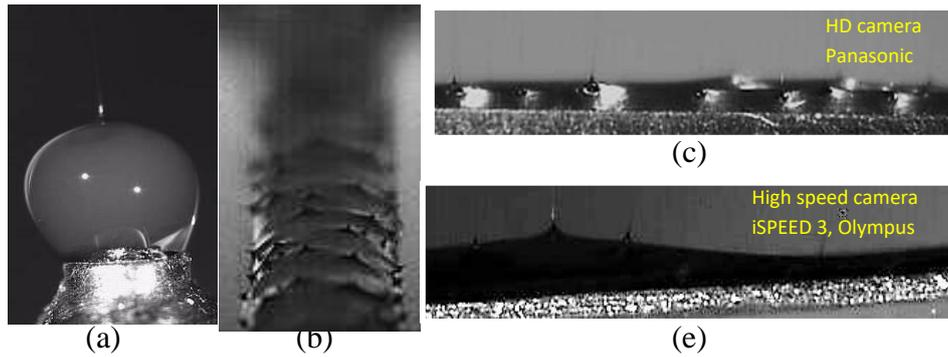
**Figure 8** Polymer jets during electrospinning realized by (a) the coaxial needle spinning electrode, (b) the cleft electrode, (c, d) the weir spinner of the 2<sup>nd</sup> generation (Valtera 2014; Vysloužilová 2015)
