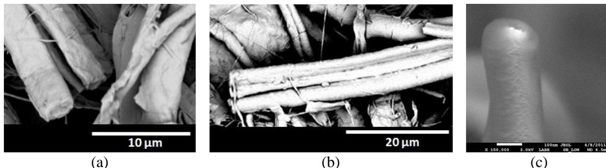
**Figure 22** Core-shell nanofibers PVA (shell) - CMC/PEO (core) analyzed by cryogenic mill by Retsch (Germany) and observed by SEM Phenom (FEI) (a, b) and core-shell nanofibers PCL (shell) and CMC (core) observed by Jeol (Germany). The core part has white color and the shell one has grey color (c), (Vysloužilová, L., 2011).
