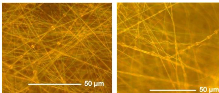
**Figure 13** Core-shell nanofibers with incorporated vegetable oil realized using electrically non-conductive material observed using optical microscope Olympus.
