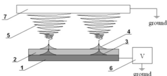
**Figure 14** The schema of the needleless coaxial electrospinning from the free surface of the polymeric two-layer: Layer of the core polymer (1), layer of the shell polymer (2), Taylor cones (3, 4), the polymer jet (5), HV supply (6), grounded collector (7), (Vysloužilová, 2010).
