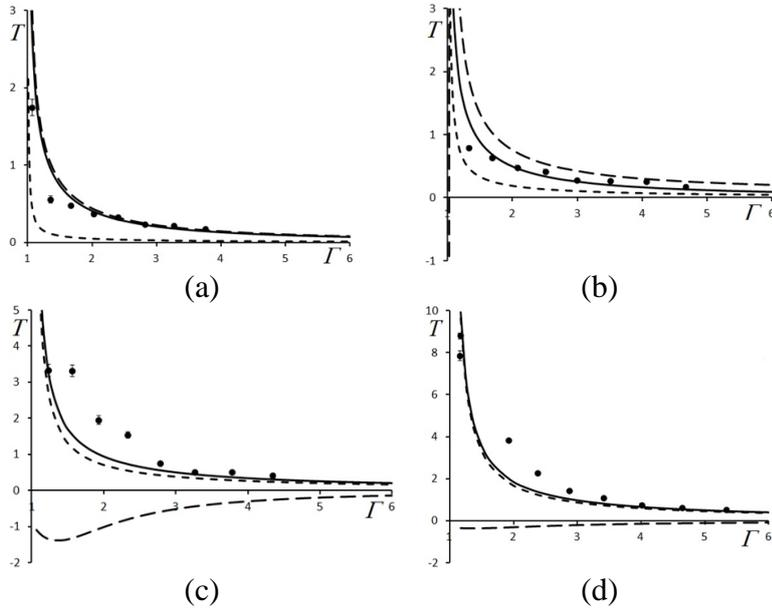
**Figure 20** The time delay  $T$  as a function of electrospinning number  $\Gamma$ . Experimental data points correspond to the mean values averaged over 10 measurements each. (a) PVA solution at concentration of 5 % (w/v),  $Oh = 0.033$ , (b) PVA solution at concentration of 8 % (w/v),  $Oh=0.132$ , (c) PVA solution at concentration of 12 % (w/v),  $Oh=0.628$  (d) PVA solution at concentration of 15 % (w/v),  $Oh=1.640$ .
