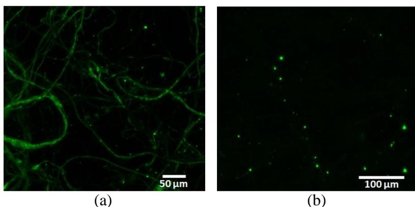
**Figure 29** Core-shell nanofibers of PCL/PVA with FITC-Dextran (a) and core-shell nanofibers of PCL/PVA with FITC-Dextran incorporated in liposomes (b). Collaboration with Andrea Míčková).
