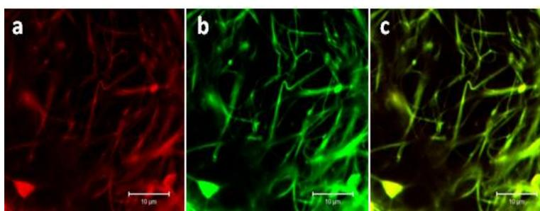
**Figure 27** Core-shell nanofibers with incorporated FITC-dextran in the shell (green signal) and Rhodamine B with IgG-PE-AF700 (red signal) in the core observed using confocal fluorescent microscopy Zeiss LSM 5 DUO: (a) the core, (b) the shell, (c) observing realized with two lasers to analysis of core-shell structure. Collaboration with Matej Buzgo (2<sup>nd</sup> Faculty of Medicine, Charles University in Prague)
