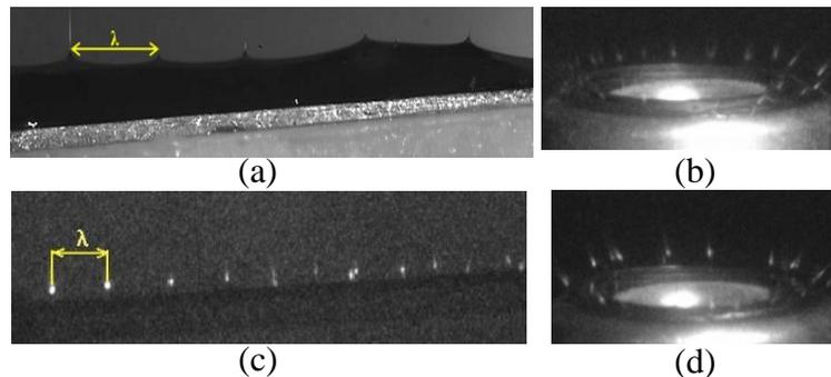
**Figure 9** The characteristic wavelength  $\lambda$  in case of needleless electrospinning recorded by (a) the high speed camera and (b-d) the UV camera (Vyslouzilova, 2015)
