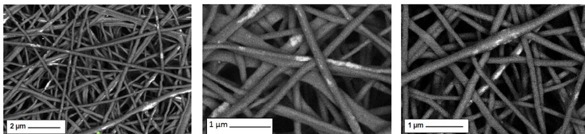
**Figure 26** SEM images of the core-shell nanofibrous structures with incorporated Prussian Blue observed by Pavel Kejzlar, KMT, FS, TUL(Zeiss, GE), (Vysloužilová, 2013).
