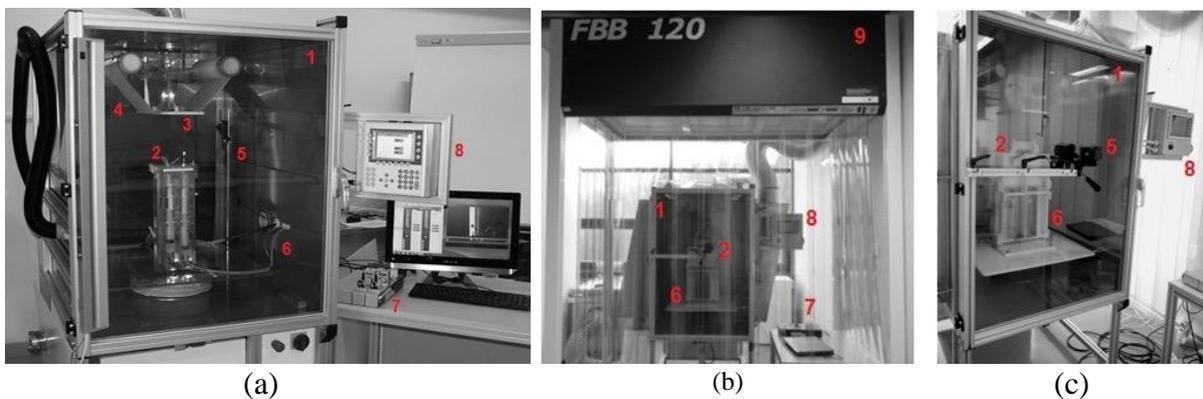
**Figure 2** Equipment for industrial production of nanofibers and core-shell nanofibers developed within this work and cluster Nanoprogres: (a) Spinner 1, (b, c) Spinner 2 for clean rooms: The coaxial equipment (1), the coaxial spinner in the holder (2), the collector (3), a nonwoven spun-bond material to collect nanofibers (4), a camera (5), a hydraulic dosing system (6), dosing syringes (7), a control panel (8), a laminar flow box (9).
