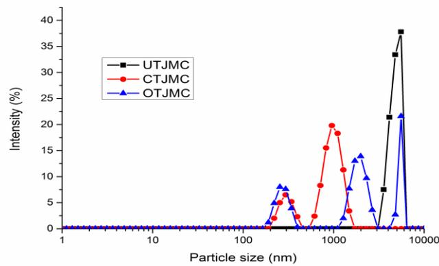
Figure 15. Particle size distribution of jute micro crystals
