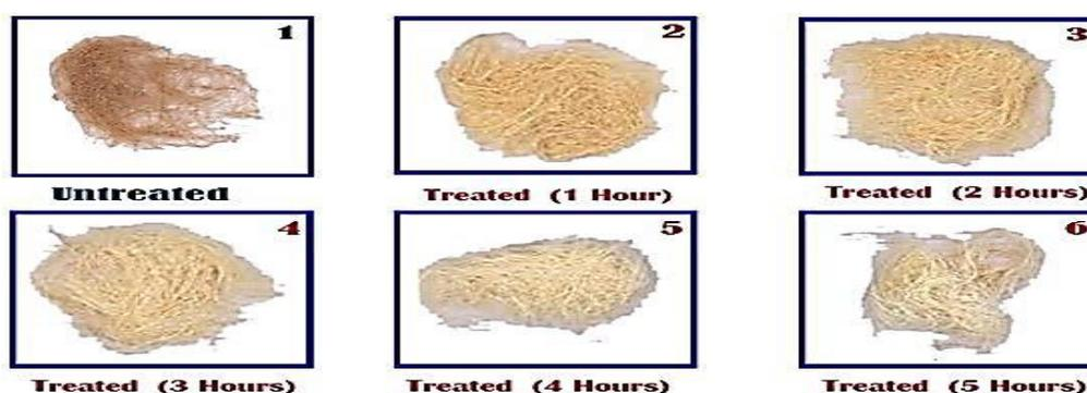
Figure 6. Apparent change in color of untreated and Ozone treated samples of jute
