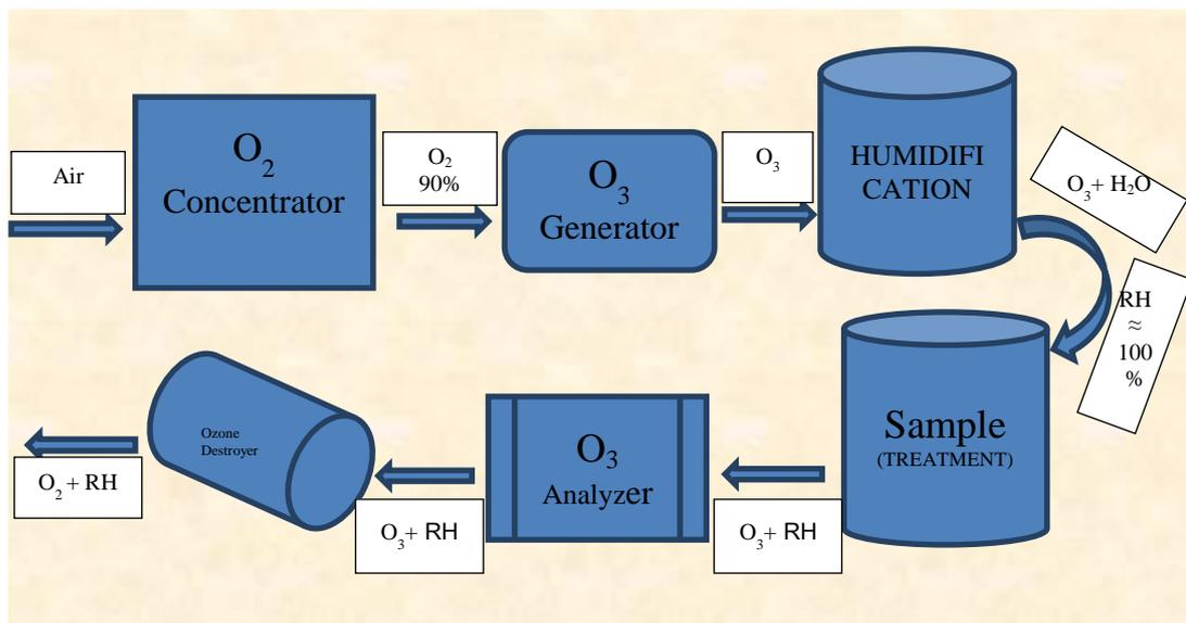
Figure 5. Schematic diagram of the Ozone Treatment Setup.
