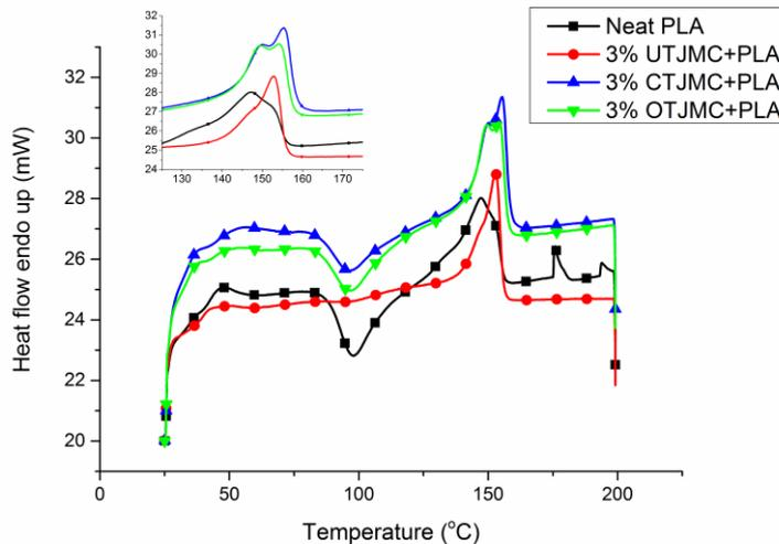
Figure 17. Differential scanning calorimetry of neat and composite PLA films
