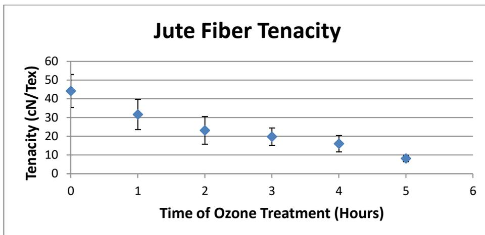
Figure 8. Decreasing trend of Tenacity with ozone treatment time (Error Bars =  $\pm 2\delta$ )
