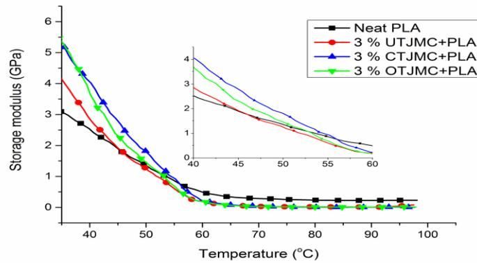
Figure 18. Storage modulus of neat and composite PLA films
