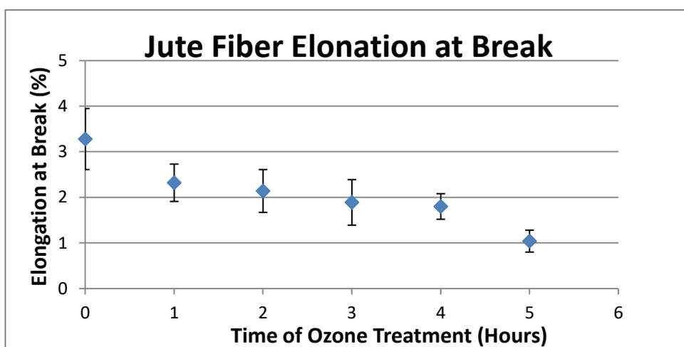
Figure 9. Elongation at Break (%) with Ozone treatment time (Error Bars =  $\pm 2\delta$ )
