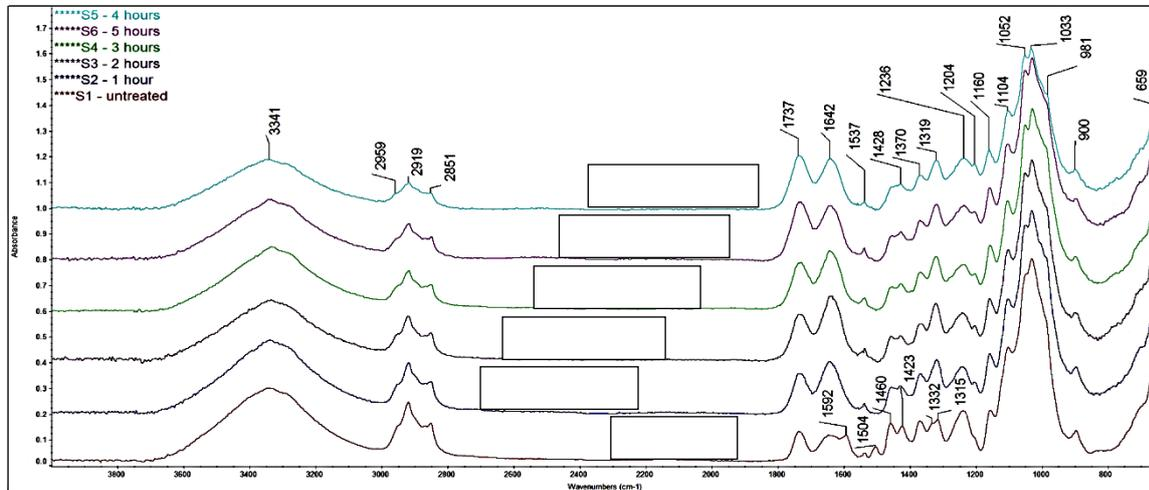
Figure 7. FTIR Spectra of Untreated and Ozone treated Jute samples
