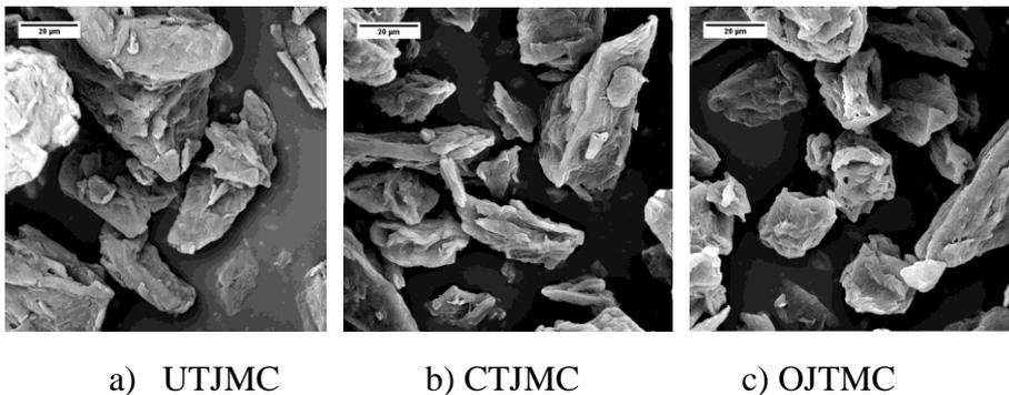
Figure 16. SEM images of Jute Micro Crystals obtained by Enzyme Hydrolysis
