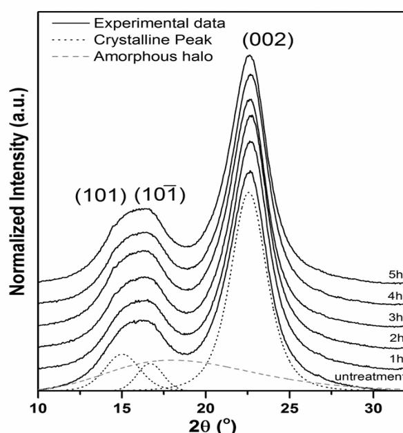
Figure 10. X-ray Diffraction Profiles of Untreated and Ozone Treated Samples of Jute Fiber
