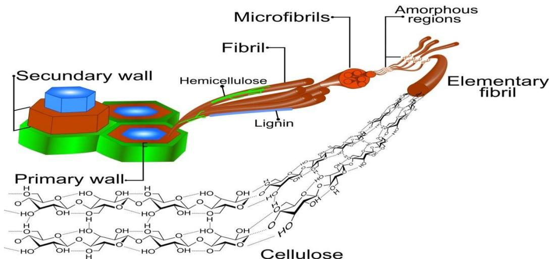
Figure 2. Hierarchical structure of cellulose extracted from plants [14]
