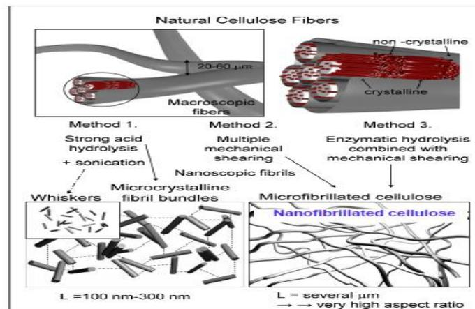
Figure 4. Types of cellulose nanostructures [32]
