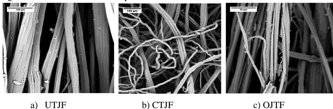
Figure 12. SEM image of Different Jute fibers used for Enzymatic Hydrolysis
