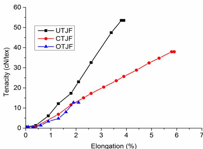
Figure 14. Single fiber strength of untreated and pre-treated jute fibers
