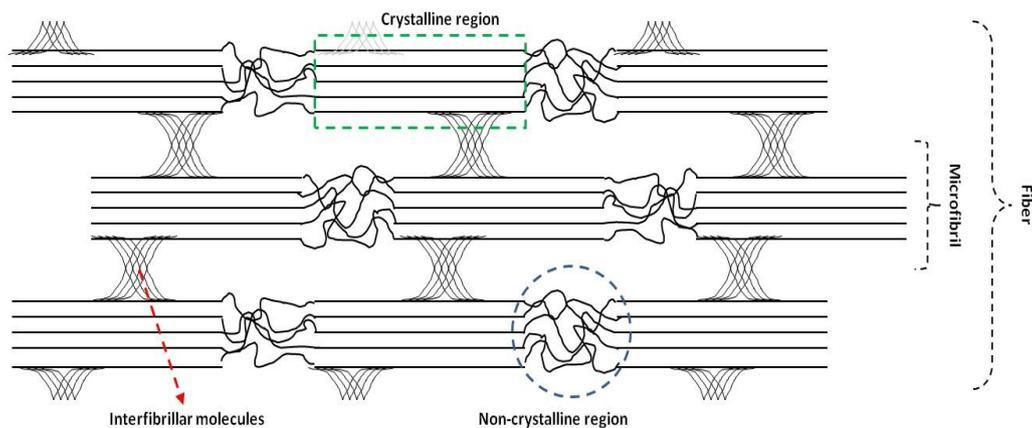
**Figure 3. Arrangement of cellulose molecules in fiber [16]**
