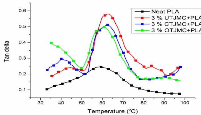
Figure 19. Damping factor of neat and composite PLA films
