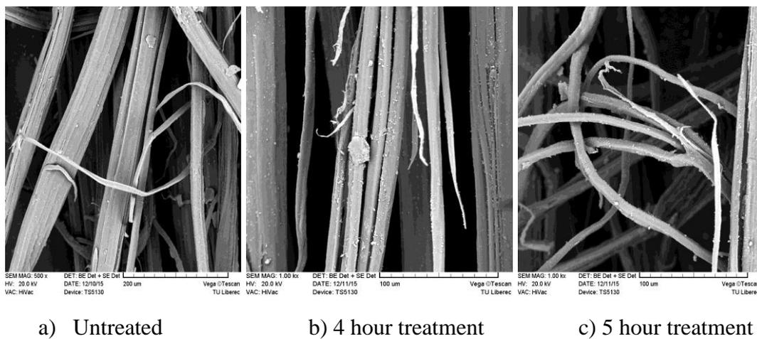
Figure 11. SEM Images of Untreated and Ozone Treated Samples of Jute Fiber
