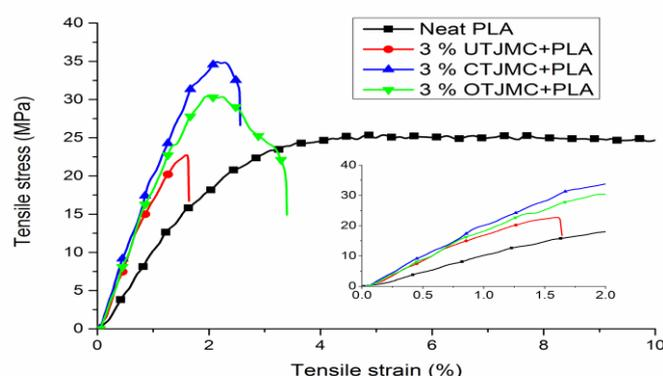
**Figure 20. Stress-strain curve of neat and composite PLA films**
