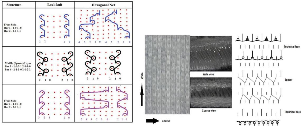
**Figure 1. Structure and knit pattern of warp and weft knit spacer fabrics**
