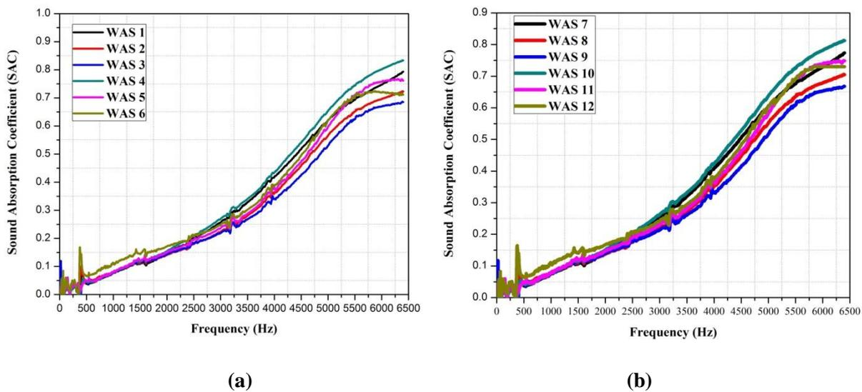
**Figure 40. Effect of structural properties on sound absorption behavior of warp knit spacer fabrics**
