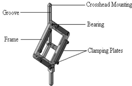
**Figure 2. Picture frame fixture design**
