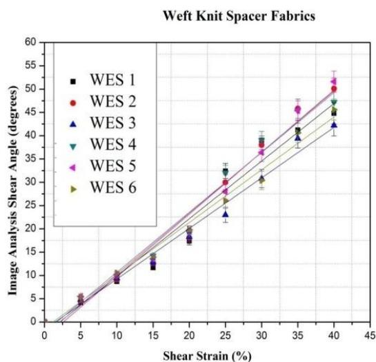
Figure 18. Linear regression fit of shear angle using image analysis as a function of strain of weft knit spacer fabrics
