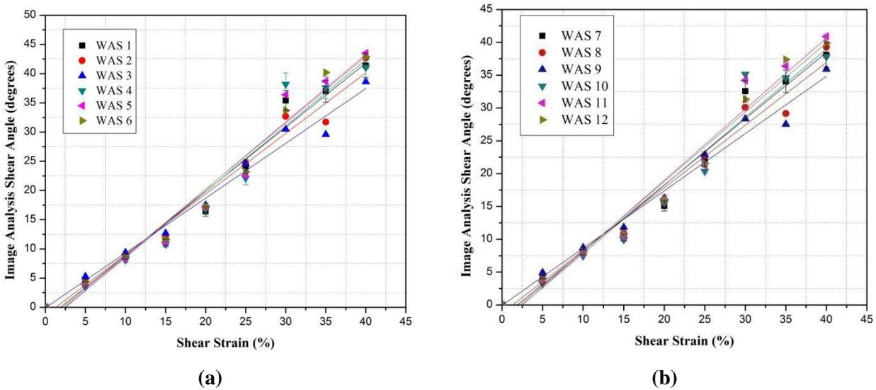
**Figure 11. Linear regression fit of shear angle using image analysis as a function of strain of warp knit spacer fabrics (a) Lock knit structure (b) hexagonal net structure**
