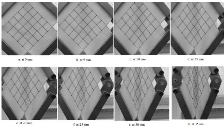
**Figure 6. Shear deformation of specimen at different displacement levels**
