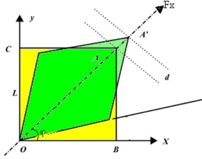
**Figure 4. Deformation kinematics of picture frame.**
