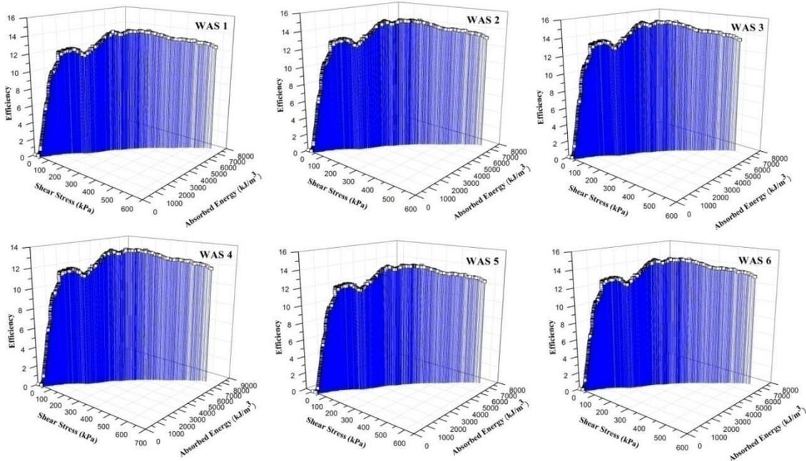
**Figure 8. In-plane shear energy absorption and efficiency of lock knit spacer fabrics**
