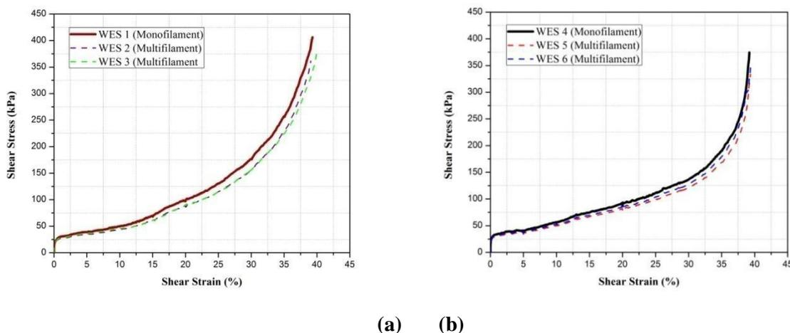
**Figure 15. Influence of fabric characteristic on shear behavior of weft knit spacer fabrics**
