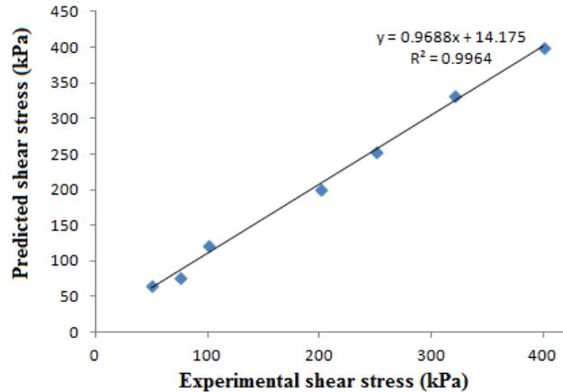
Figure 21. Correlation of shear stress predicted vs experimental
