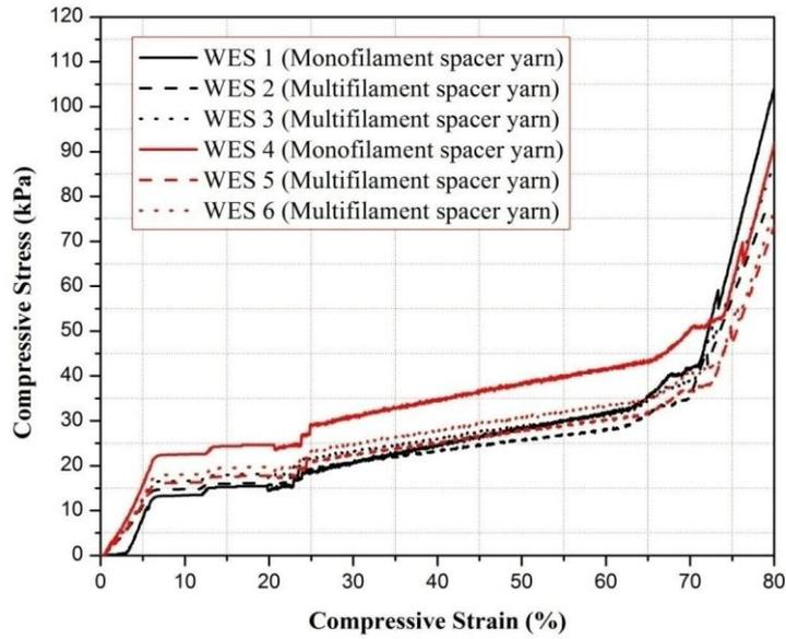
**Figure 27. Influence of fabric characteristics on compressive behavior of weft knit spacer fabrics**
