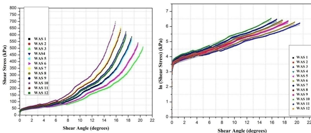
**Figure 10. Experimental determination of shear angle vs shear force and linear regression fit of warp knit spacer fabrics**
