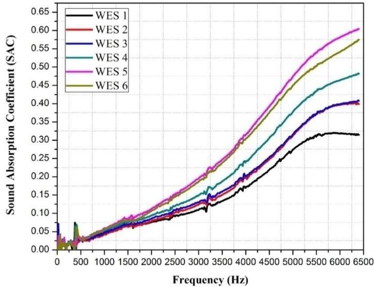
Figure 43. Effect of structural characteristics on sound absorption behavior of weft knit spacer fabrics
