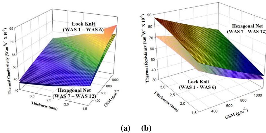
**Figure 32. Effect of gsm and thickness on thermal properties of warp knit spacer fabrics**
