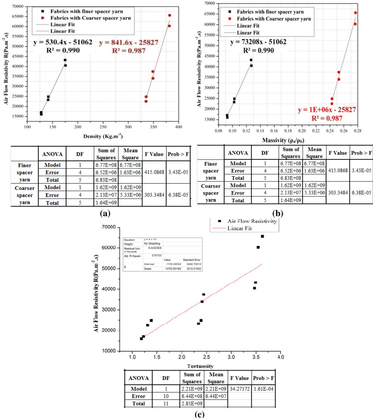
Figure 39. Effect of structural characteristics and linear regression model for air flow resistivity of warp knit spacer fabrics
