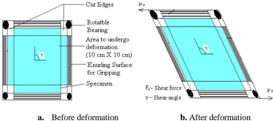
**Figure 3. Shear deformation of frame and specimen**
