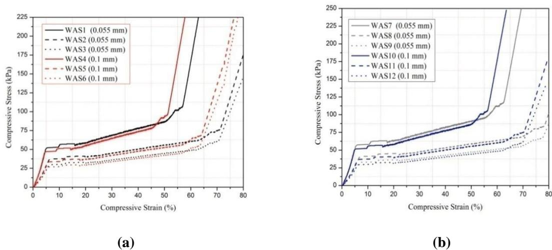
**Figure 22. Influence of thickness and spacer yarn on compressive behavior of warp knit spacer fabrics**
