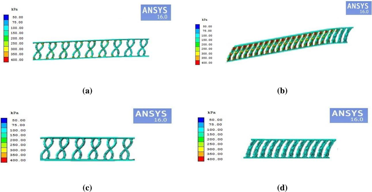
Figure 20. Weft knitted spacer (a) without Lycra before shear (b) without Lycra after shear (c) with Lycra before shear and (d) with Lycra after shear
