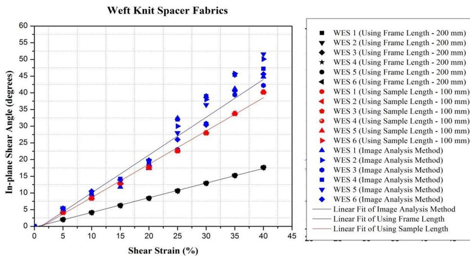
Figure 19. Comparison of shear behavior of weft knit spacer fabrics using different test methods
