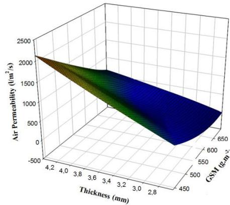
Figure 35. Influence of structural parameters on air permeability of weft knit spacer fabrics
