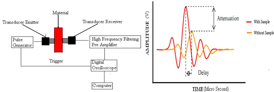
**Figure 5. Experimental set up to measure tortuosity using ultrasonic method.**
