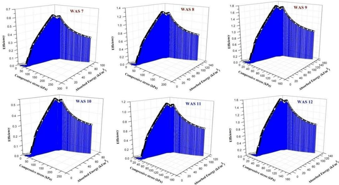
Figure 25. Energy absorption and efficiency of hexagonal net spacer fabrics
