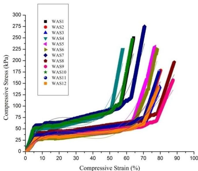
**Figure 26. Third order polynomial regression fit for compressibility of warp knit spacer fabrics**
