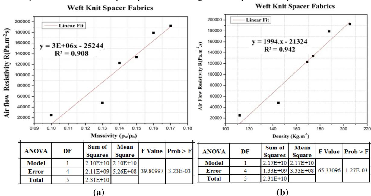
**Figure 42. Effect of structural characteristics and linear regression model for air flow resistivity of weft knit spacer fabrics**
