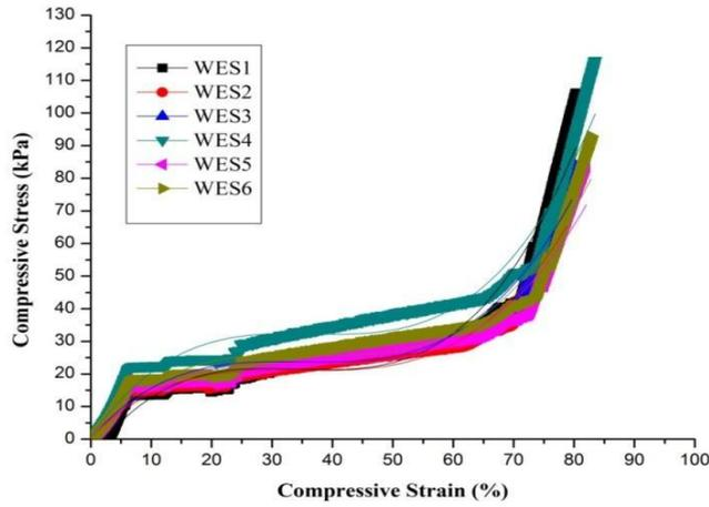
Figure 29. Third order polynomial regression fit for compressibility of weft knit spacers
