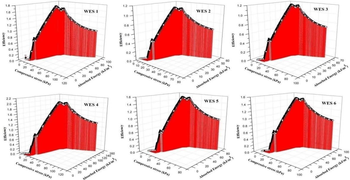
**Figure 28. Energy absorption and efficiency of weft knit spacer fabrics**
