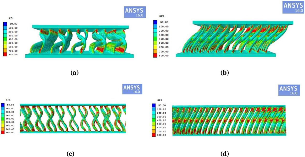
**Figure 13 (a) Lock knit spacer before shear, (b) Lock knit spacer after shear, (c) Hexagonal net spacer before shear and (d) Hexagonal net spacer after shear**
