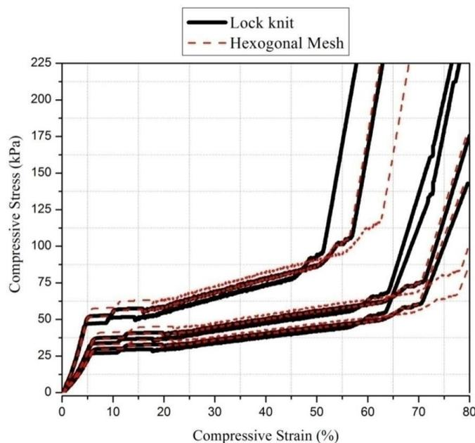
**Figure 23. Influence of surface structure on compressive behavior of warp knit spacer fabrics**
