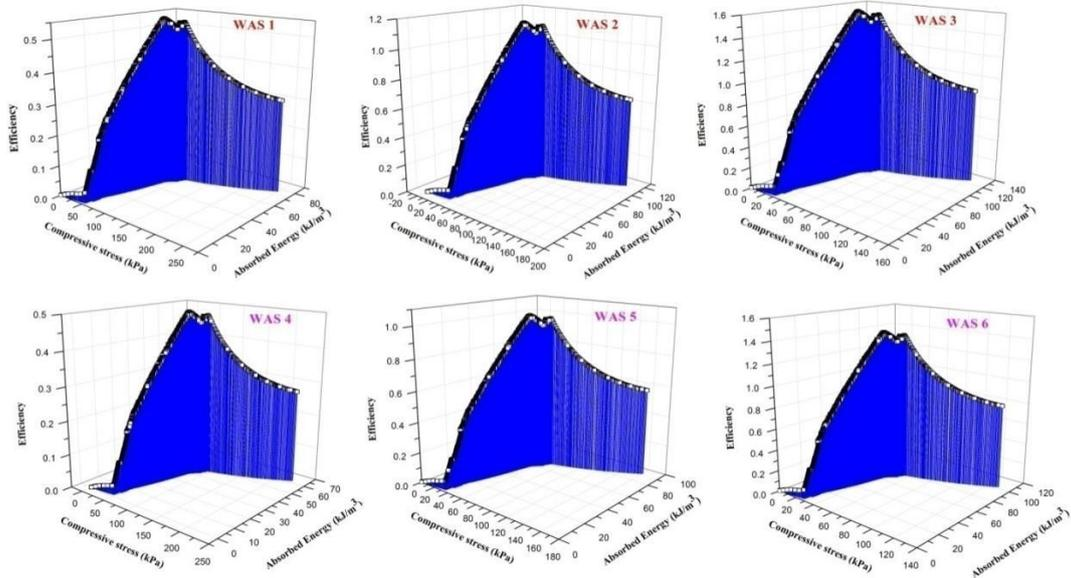
Figure 24. Energy absorption and efficiency of lock knit spacer fabrics
