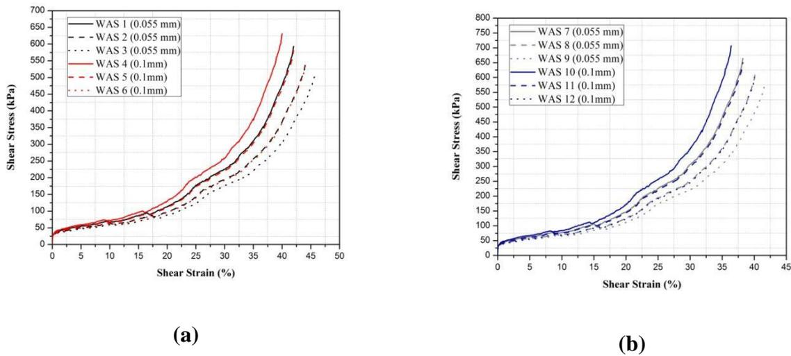
**Figure 7. Influence of spacer yarn linear density on shear behavior of warp knit spacer fabrics (a) Lock Knit, (b) Hexagonal Net**
