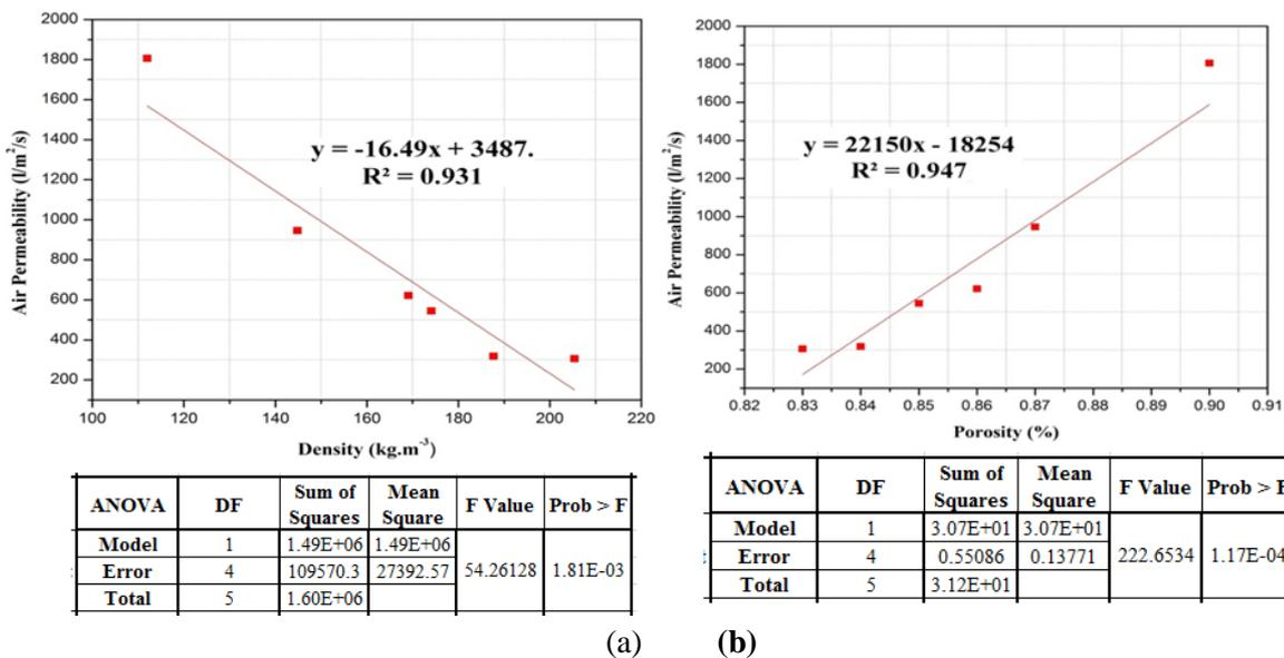
Figure 36. Effect of structural characteristics and linear regression model for air permeability of warp knit spacer fabrics
