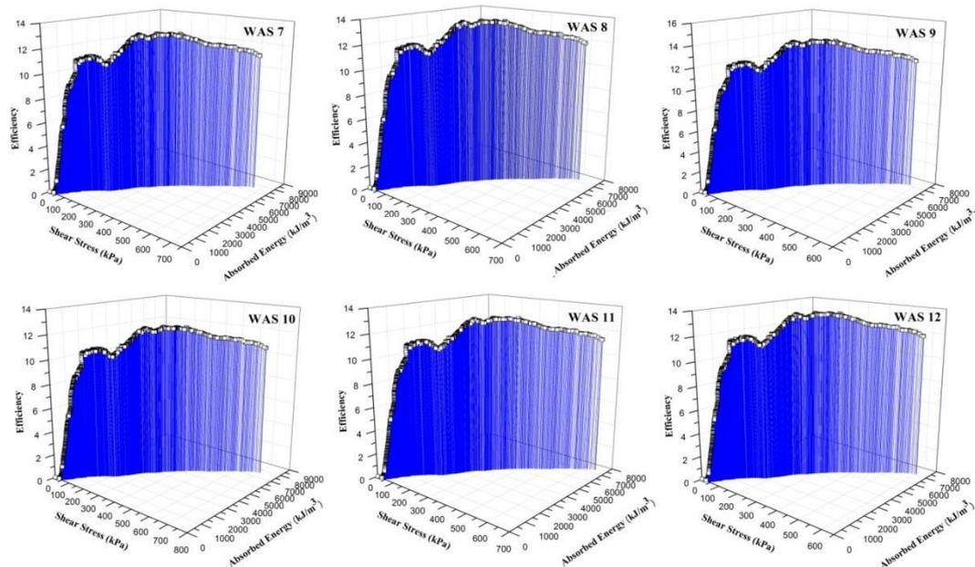
**Figure 9. In-plane shear energy absorption and efficiency of hexagonal net spacer fabrics**
