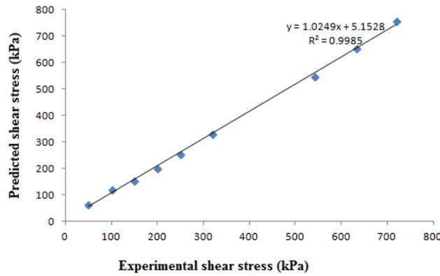
**Figure 14 Correlation of simulated and experimental shear stress**
