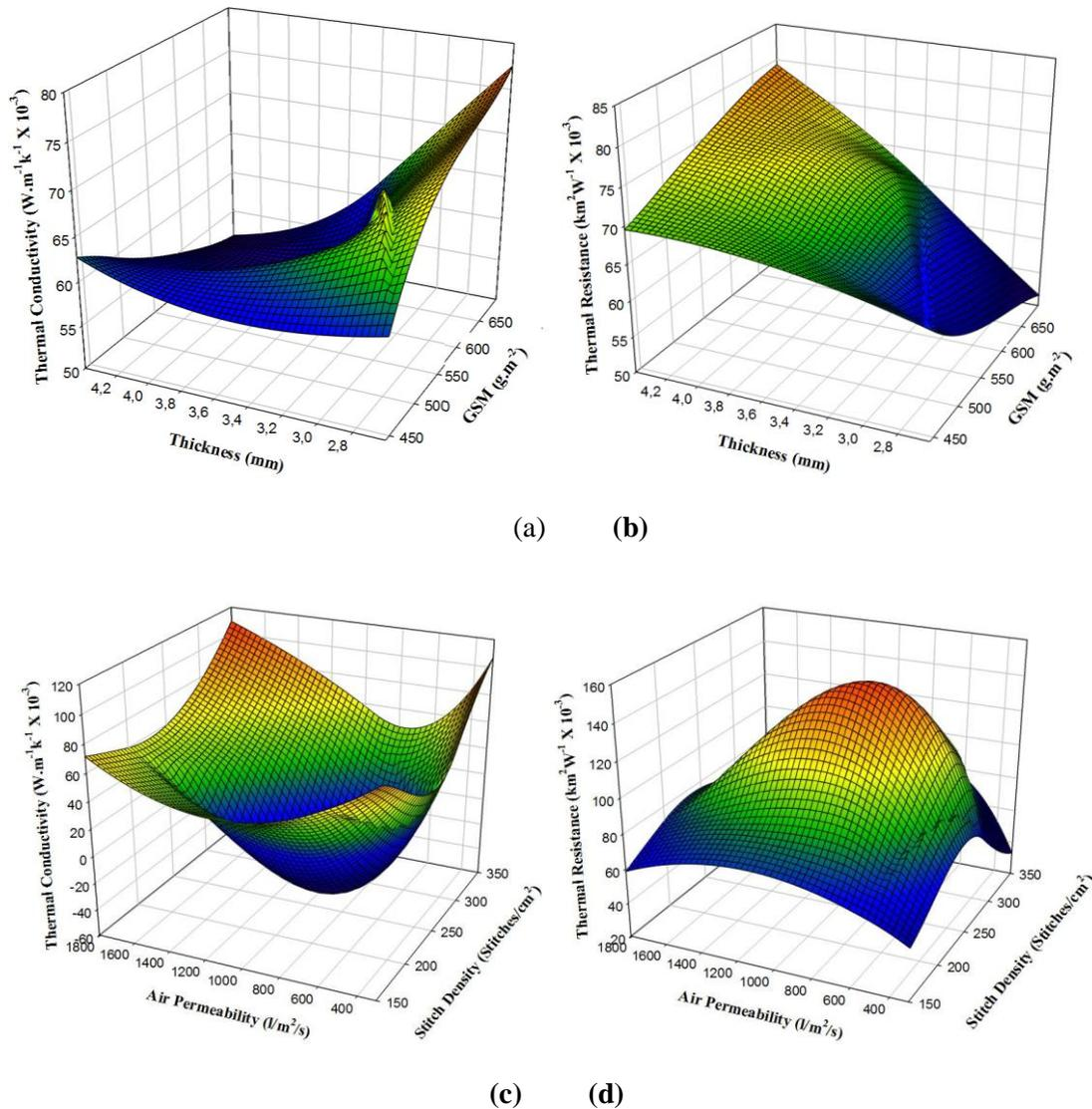
**Figure 37. Influence of structural parameters on thermal properties of weft knit spacer fabrics**
