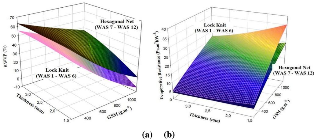
**Figure 33. Effect of thickness and areal density on water vapour permeability**
