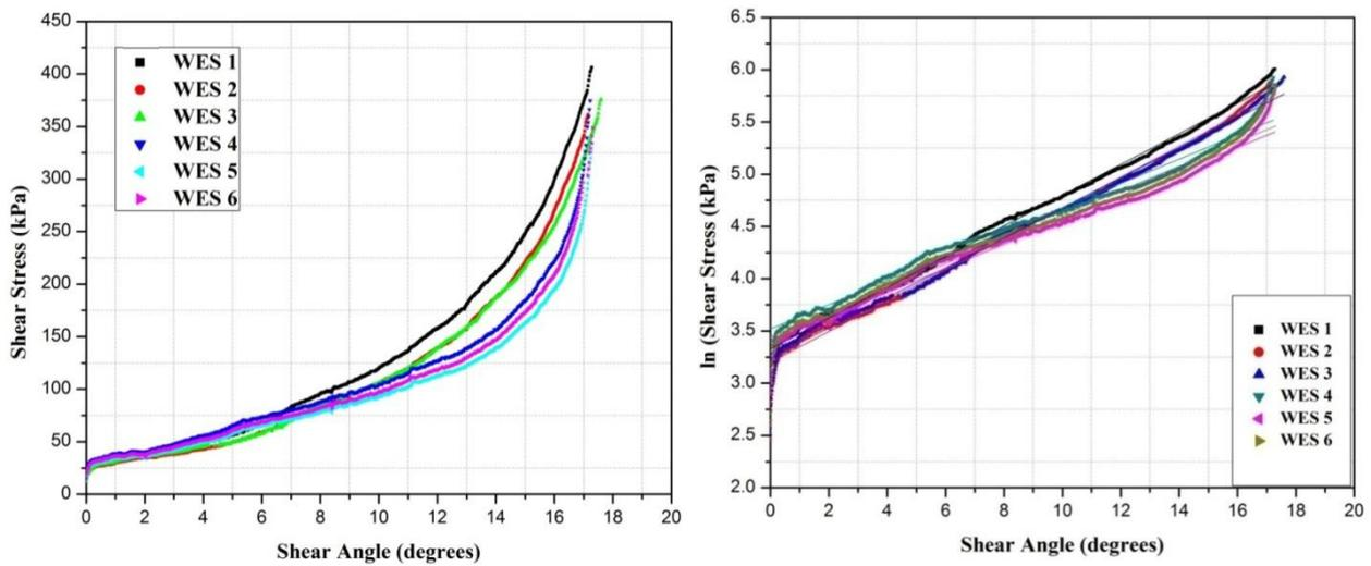
Figure 17. Experimental determination of shear angle vs shear force and linear regression fit of weft knit spacer fabrics
