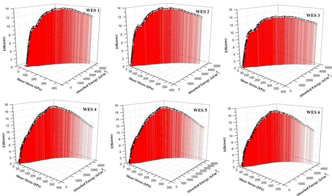
Figure 16. In-plane shear energy absorption and efficiency of weft knit spacer fabrics
