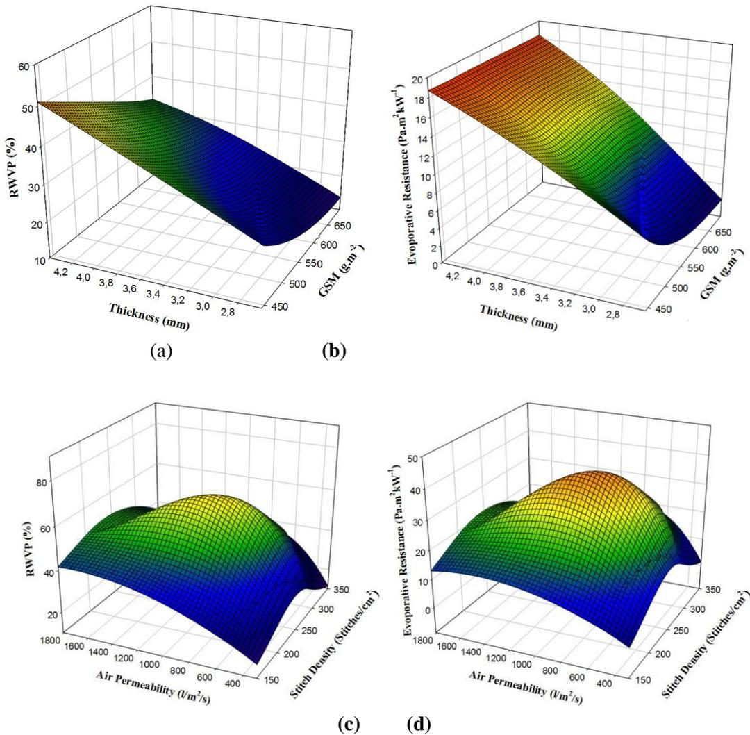
**Figure 38. Influence of structural parameters on thermal properties of weft knit spacer fabrics**
