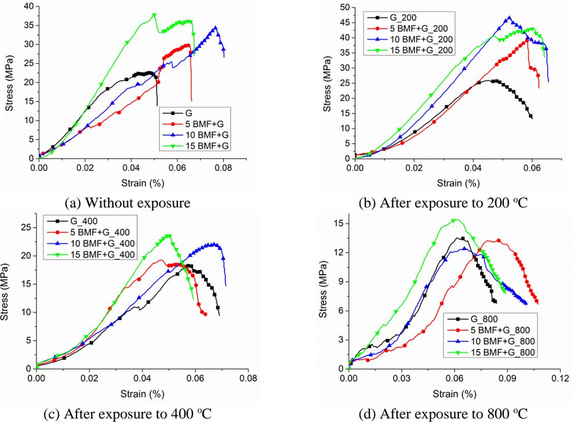
Figure 12. Stress-strain curve for BMF/geopolymer composites
