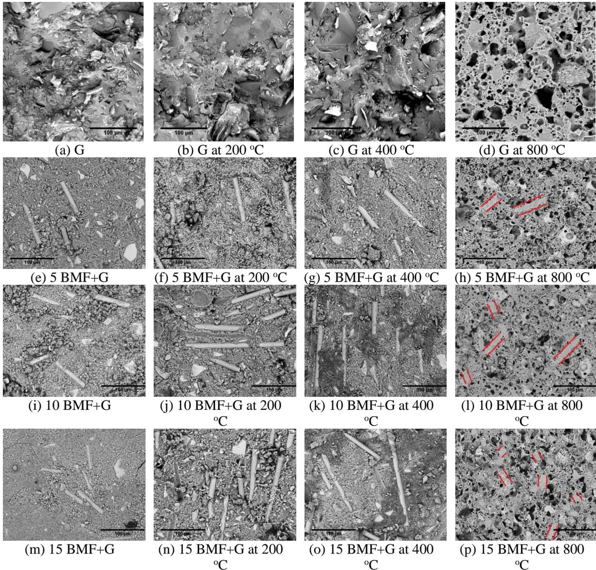
Figure 5. Microstructure of basalt microfibril/geopolymer composites at elevated temperature
