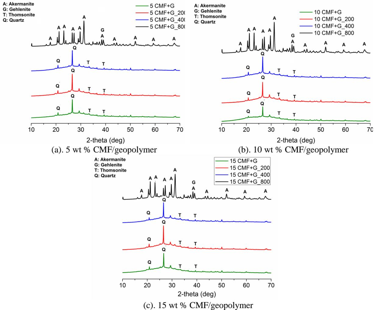
Figure 11. XRD analysis of carbon microfiber/geopolymer composites
