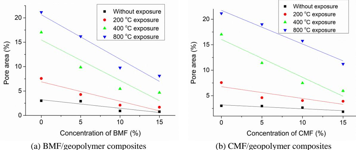
Figure 9. Estimation of pore area of geopolymer composites
