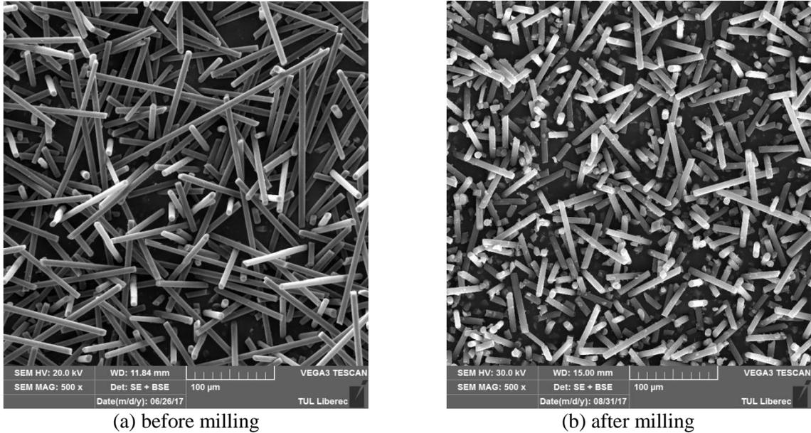
Figure 4. Microstructure of carbiso powder
