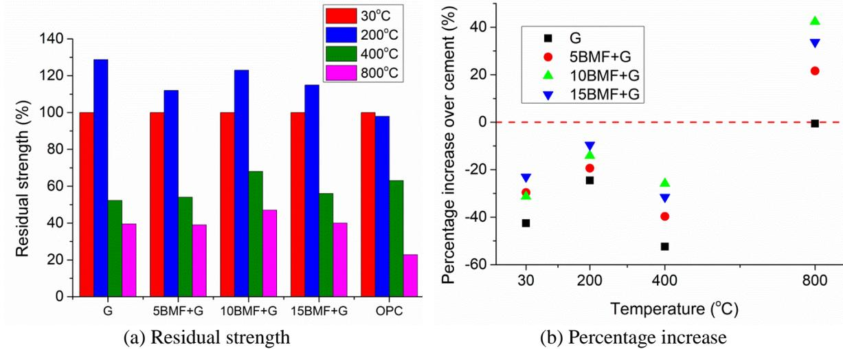
Figure 13. Compression strength comparison of BMF/geopolymer composites with OPC
