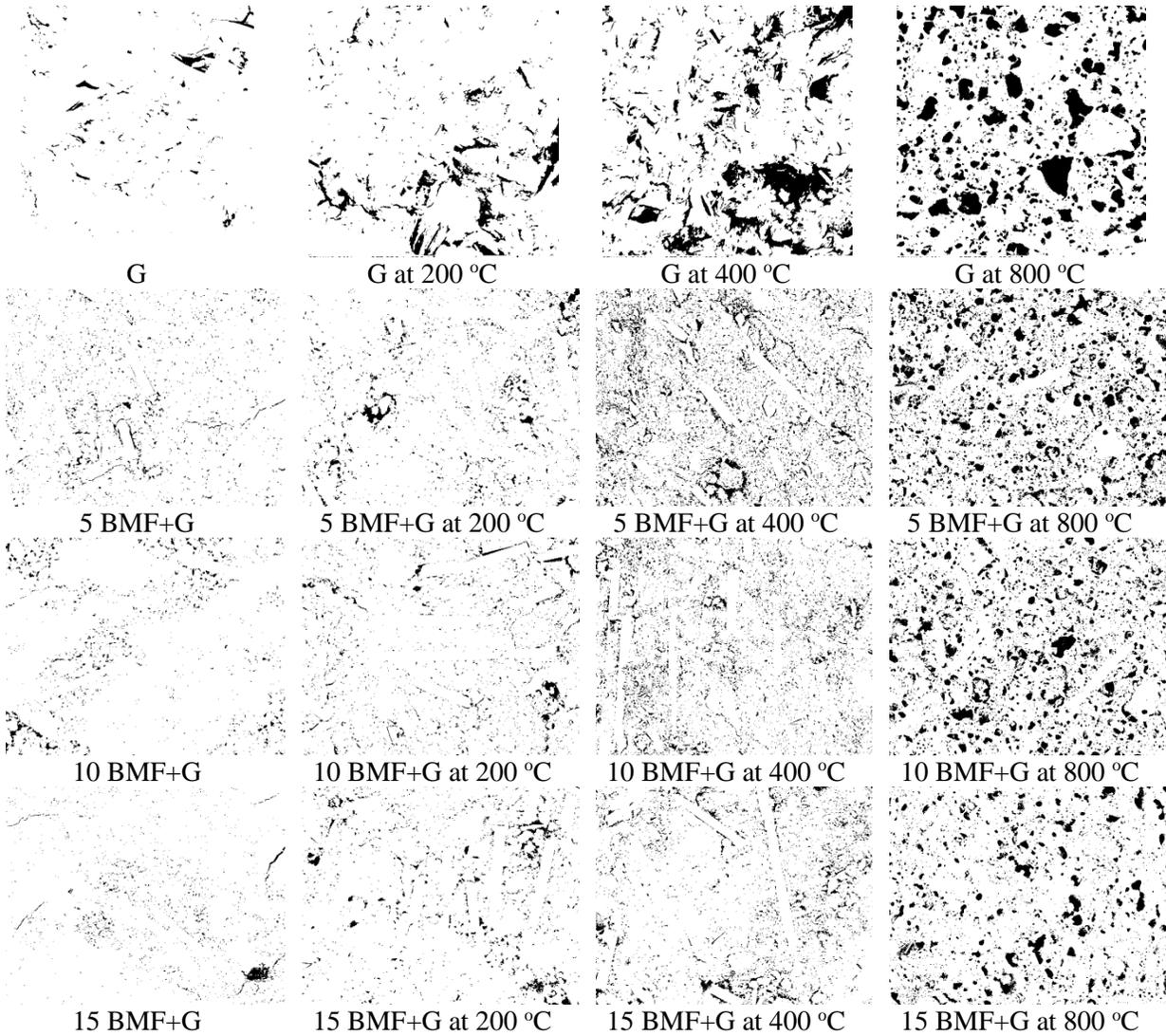
Figure 7. Estimation of pore area in basalt microfibril/geopolymer composites by image analysis
