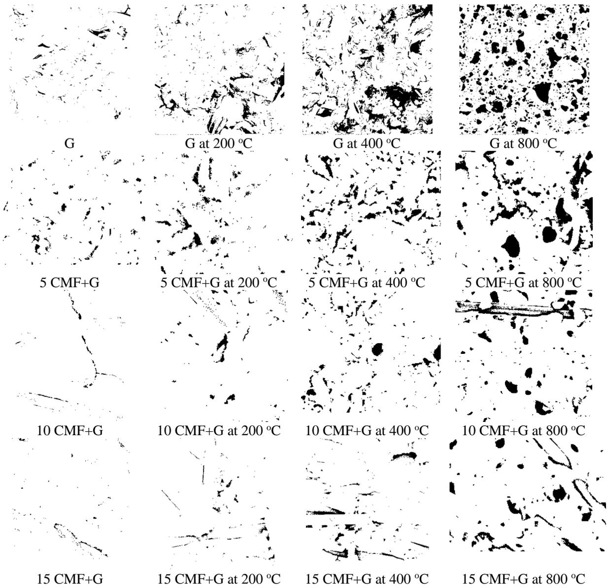
Figure 8. Estimation of pore area in carbon microfiber/geopolymer composites by image analysis
