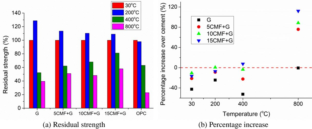
Figure 15. Compression strength comparison of CMF/geopolymer composites with OPC
