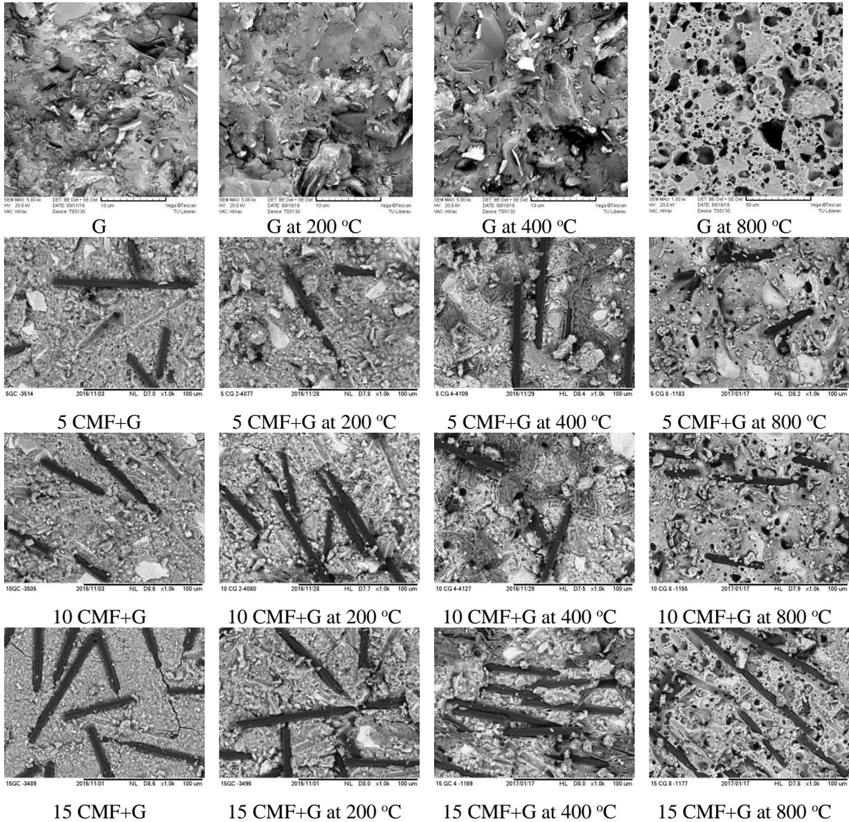
Figure 6. Typical fracture surface microstructure of carbon microfiber/geopolymer composites after exposure to elevated temperature
