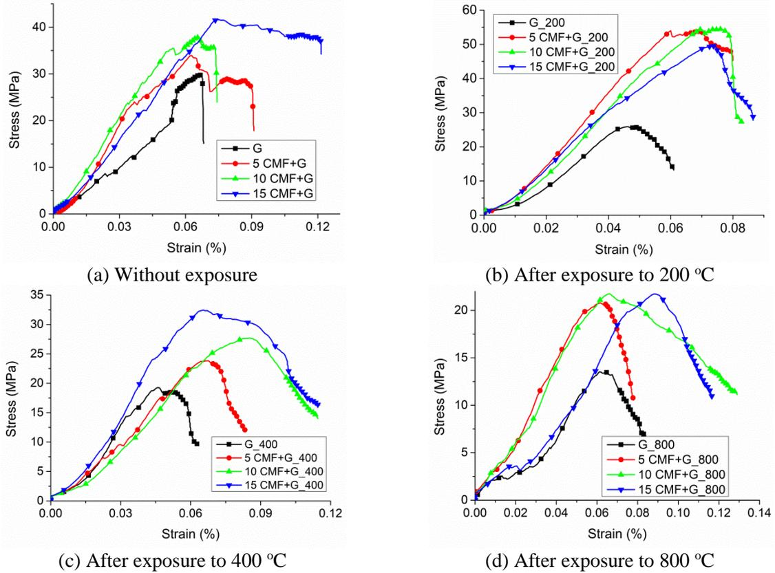
Figure 14. Stress-strain curve for CMF/geopolymer composites
