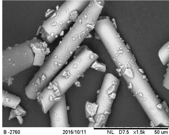
Figure 2. (a) Particle size distribution of basalt particles after 30 min dry milling (b). SEM image of basalt fibers after 30 min dry milling
