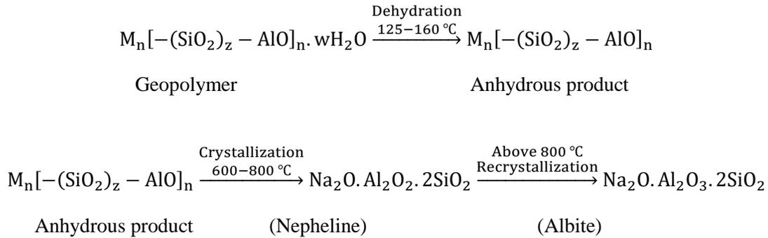
Figure 1. Geopolymer phase transformation during fire [24].
