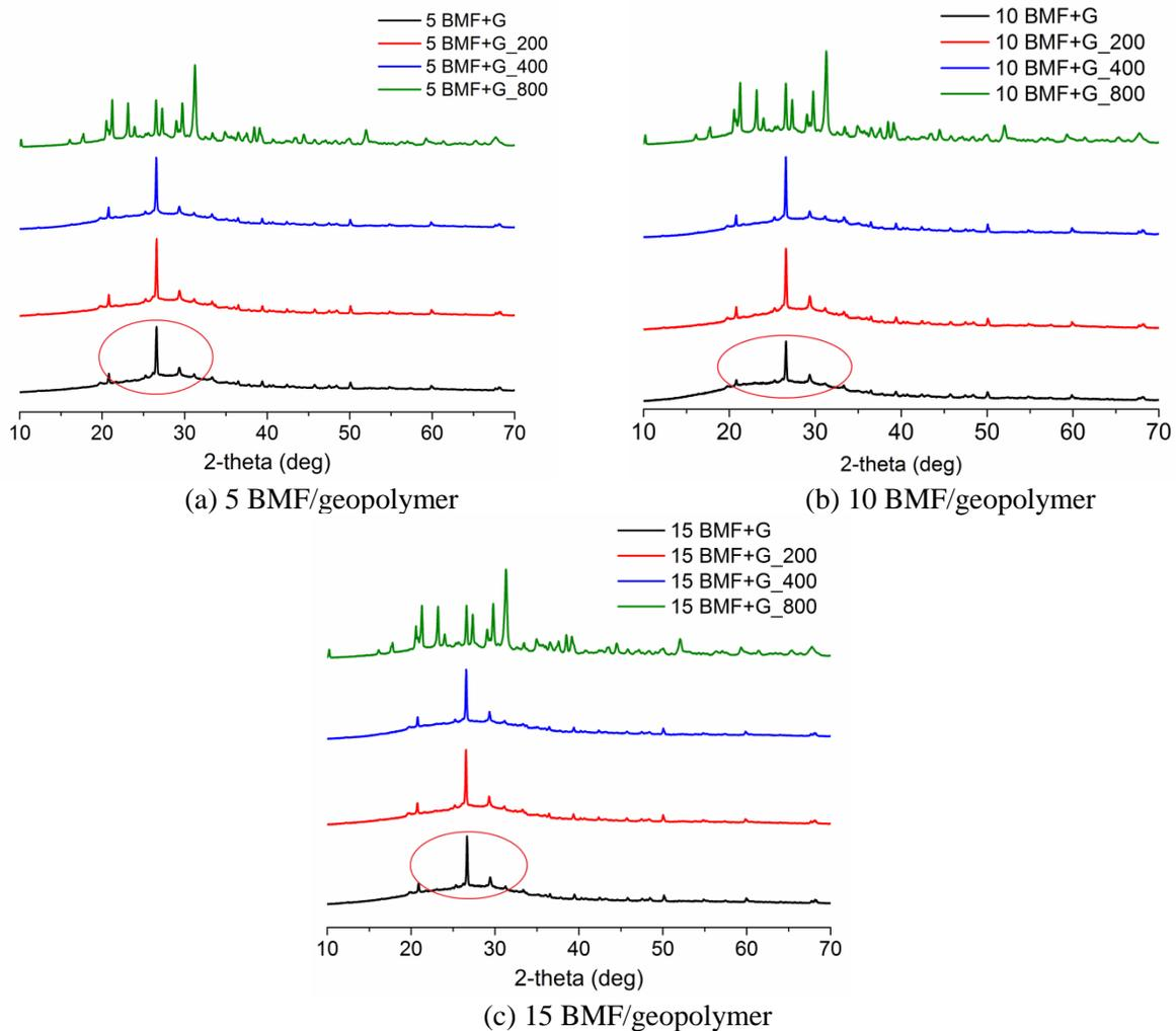
Figure 10. XRD analysis of basalt microfibril/geopolymer composites at elevated temperature
