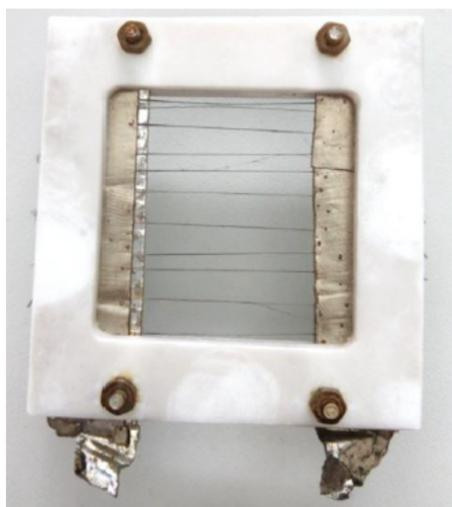
FIGURE 4.1: Polypyrrole-coated PCL fibers made by drawing, fixed within a Teflon frame in between an aluminum foil [19]
