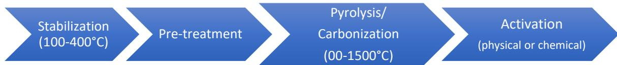
Fig. 3. Main stages involved in the production of ACFs.
