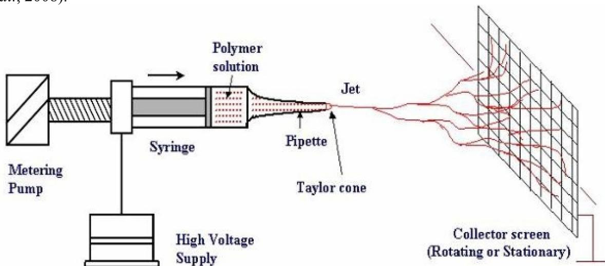
**Fig. 2.1: Schematic diagram of an electrospinning set up**
