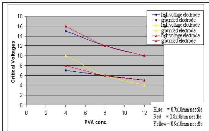
Figure 9.4 Variation of critical voltages with varying PVA conc.
