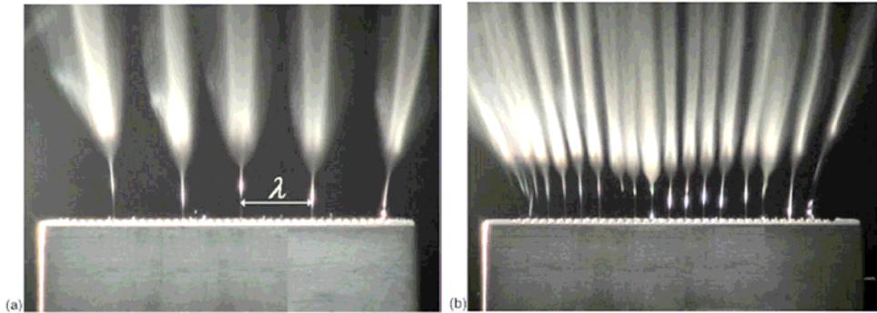
**Fig. 5.1.** Linear clefts emit polymeric jets. Clefts in (a) and (b) emit polymeric polyvinyl alcohol jets at the voltages, 32 and 43 kV, respectively. The interjet distance/wavelength is  $\lambda$ .
